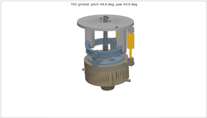
5.2 Gimbal sweep. The full 6° cone without clashing; stroke and force from the kinematic model.
